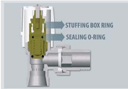
An effective seal is ensured within the valve body by means of a stuffing box with an internal O-ring, while in the lockshield valve it is achieved by two O-rings located on the stem. During assembly the two O-rings are oiled, thus creating a lubricated zone between them, which avoids shutter locking.
