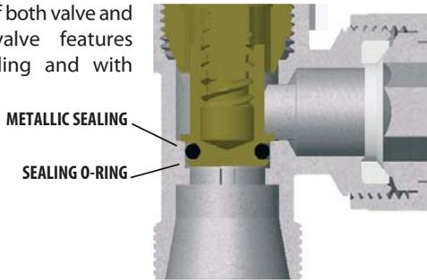
Terminals have a conical thread to optimize the seal and are provided with a special soft film - Loctite® Dri-Seal5061- which guarantees an effective seal on standard threading. If necessary, it is possible to apply the film with other common types of sealing system.
